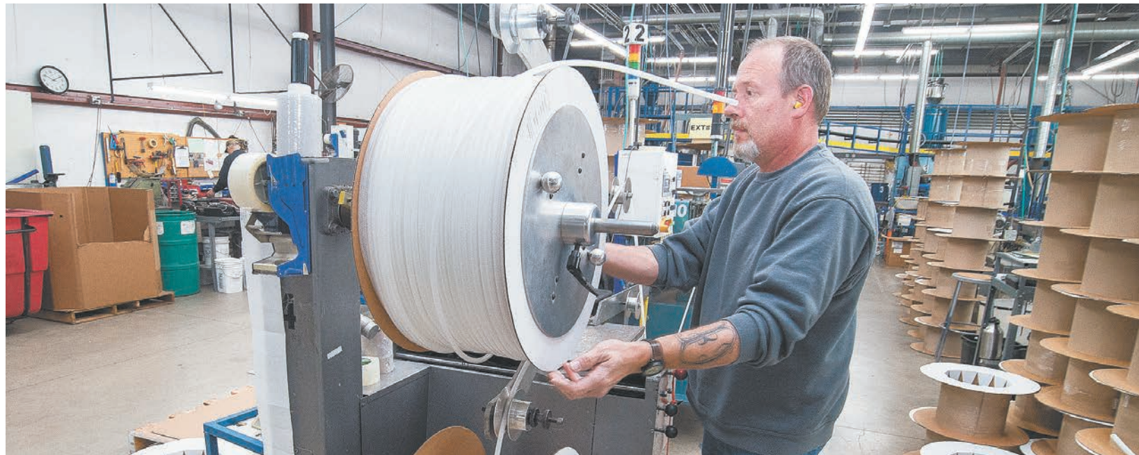
Freelin-Wade worker Rick Drahiem finishes up a spool of reinforced polyurethane tubing on the manufacturing line. The company began making medical-grade tubing this year for ventilators produced by General Motors Co. Photo by Marcus Larson
